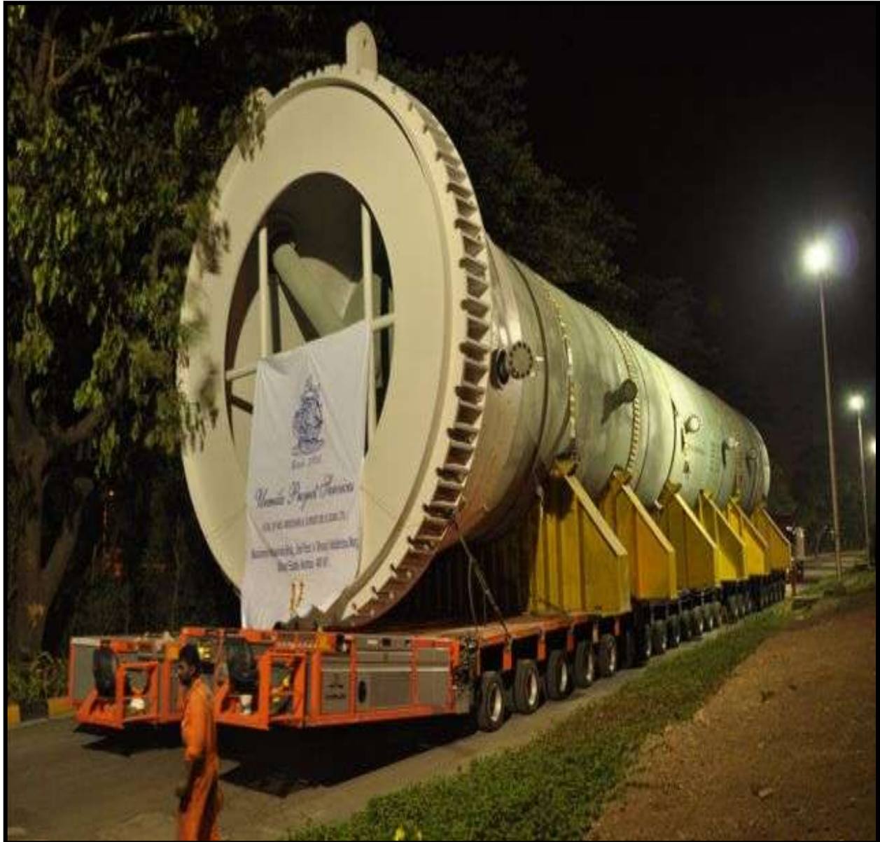
Transportation of DHDS Reactor 40m x 8.6m x 8.5m – 930 MT on 24+24 Goldhofer self-propelled axles.
