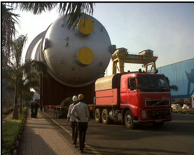
Transportation on 12+12 hydraulic axles trailer.
