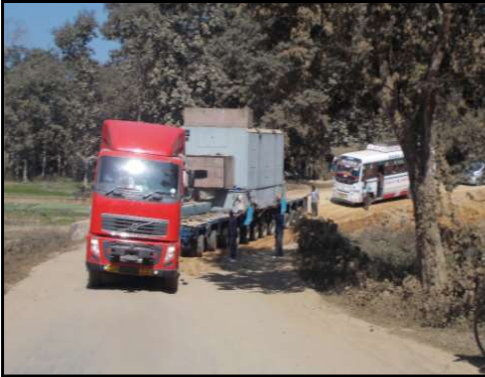
Transportation of Gas Turbine Generator 8.70m x 3.50m x 4m – 162 MT from Karimganj to Monarchak Tripura Project
