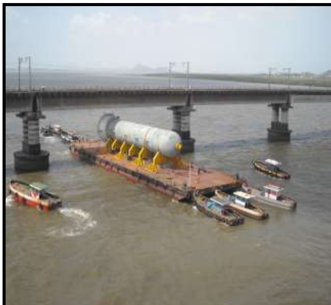
Barge loaded with DHDS Reactor 40m x 8.6m x 8.5m – 930 MT passing under the bridge at Vashi, Mumbai during voyage from Godrej & Boyce Mfg.Co.Ltd Vikhroli jetty to Mumbai port
