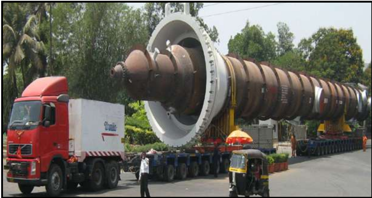
First longest package (Reactor 3 & 4 - 64.39m x 6.37m x 6.94m – 410 MT) moved out of Godrej Vikhroli factory and handled by Urmila for IOCL Paradip on Goldhofer hydraulic axles with bolster arrangement.
