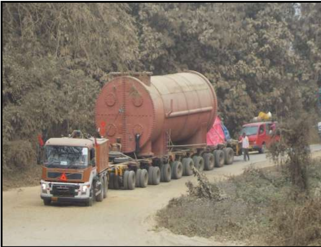
Transportation of Gas Turbine Generator 8.70m x 3.50m x 4m – 162 MT from Karimganj to Monarchak Tripura Project
